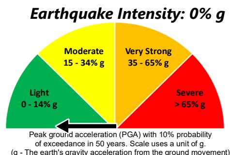
Peak ground acceleration (PGA) with 10% probability of exceedance in 50 years. Scale uses a unit of g.
