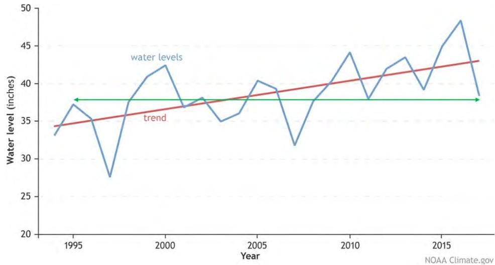
*Figure 6. Virginia Key between 1994 and 2017 has risen by more than 5 inches because of sea-level rise (red line). Water level elevations during low tide are now greater than the high tides that occurred 20 years earlier.*
