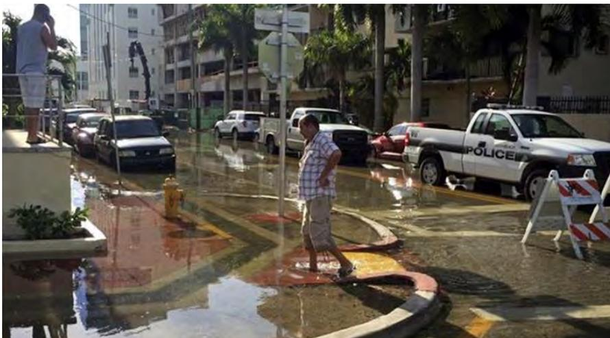
*Figure 5. Saltwater bubbling onto the street from a stormwater drain during exceptional tide event.*
