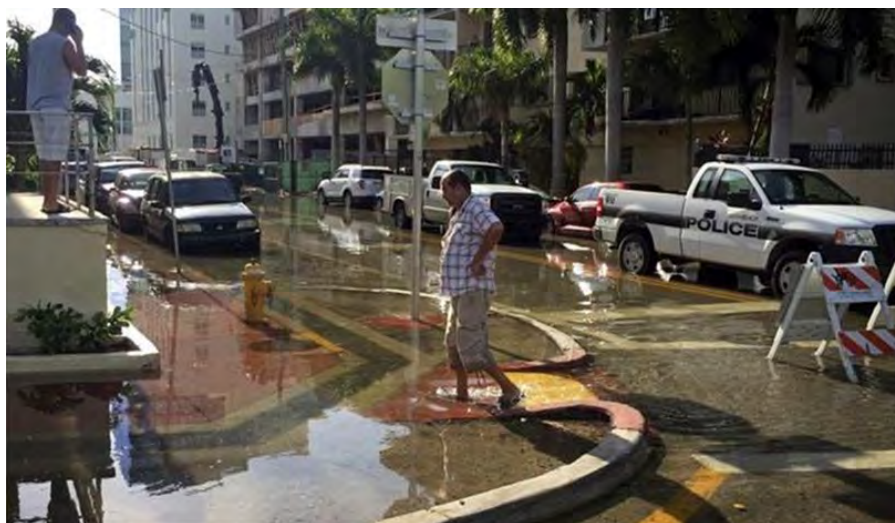
Figure 4. .When built, storm water generated during heavy rainfall drained by gravity into the ocean, even during exceptional tides (top). But because sea level has risen by more than a foot over since the 1920's salt water now flows through the aging stormwater pipes and into low-lying streets, sidewalks and yards (bottom) where it saturates the soils upon which they were constructed.
